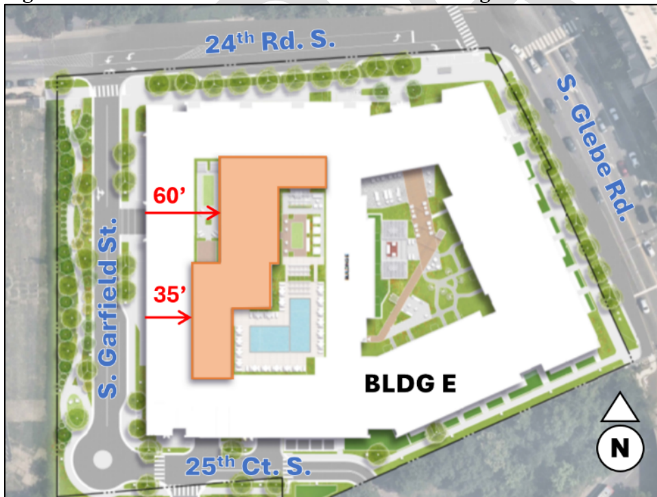
Figure 18. Penthouse Level Setbacks from Roof Edge.
