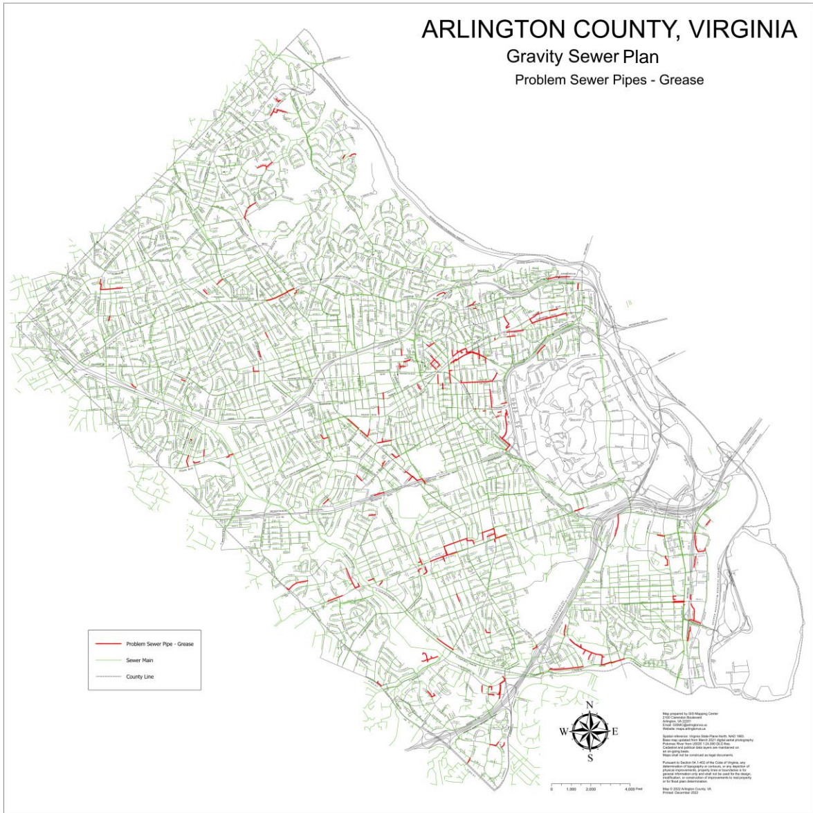
Figure 2-5 Sewer Segments Regularly Flushed to Remove Grease
